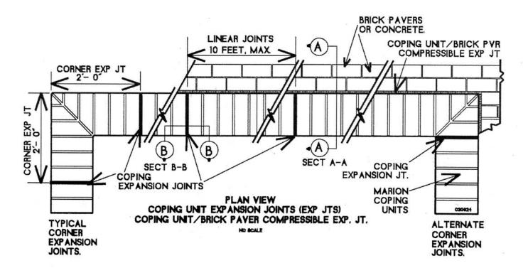
■Expansion joints through coping units shall extend through the coping unit and mortar to the bond beam (top of pool wall). See drawing below.
