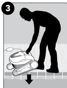
Put the Pool Cleaner into the pool. Release the Pool Cleaner and let it sink to the floor of the pool. Make sure that the floating cable is free of any obstructions.
