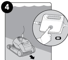
Turn the power supply ON. The Pool Cleaner will now operate until it has reached the end of the cleaning cycle.
