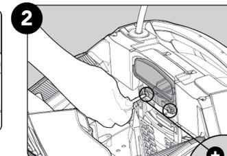
Using a short screwdriver open the 2 screws.
