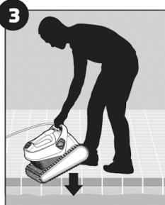
Release the Pool Cleaner and let it sink to the floor of the pool. Make sure that the floating cable is free of any obstructions.
