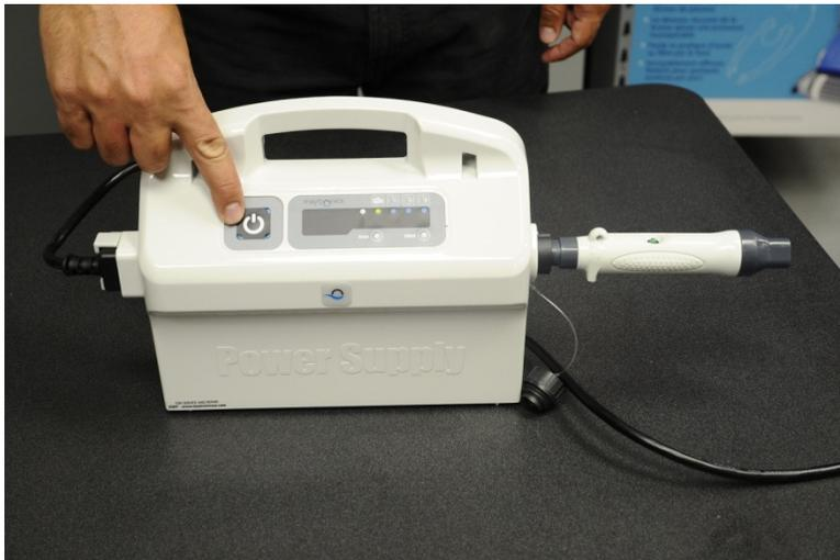
Insert round end of Dolphin tester into power supply where cable connects. Plug in power supply and push power button.
