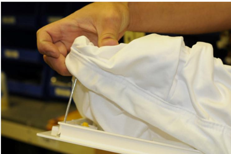
To remove the filter bag, remove black plastic clips and slide bag off of metal frame.
