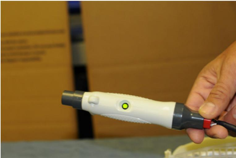
A green light indicates the cable is good. If you do not get a green light, and you are sure all connections are secure, replace cable.
