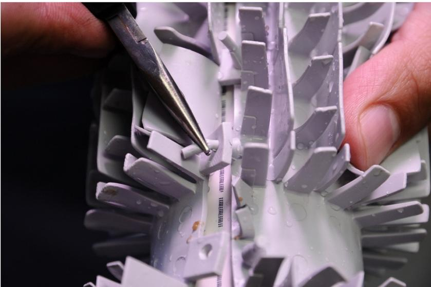
PVC brushes can be replaced by pulling the stems at the seam through the holes in the tabs using pliers. **Note: A diluted solution of dish soap can help lubricate the stems.**
