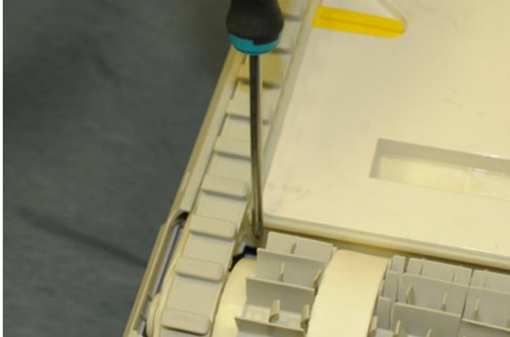
Turn the robot over and insert a screw driver between the brush and the bottom lid at the side next to the tracks.
