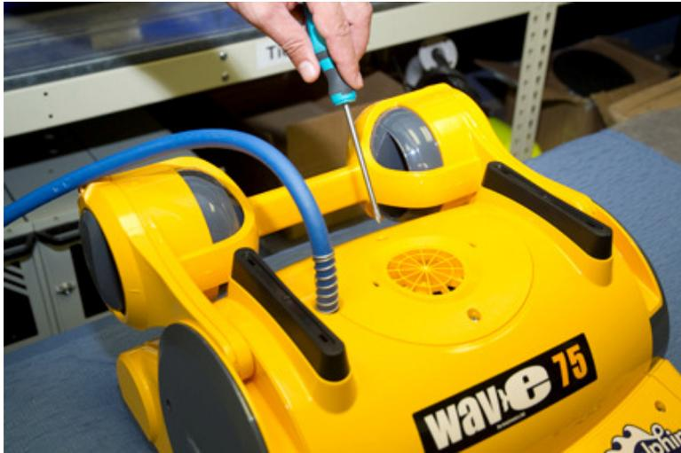
Remove screw(s) holding impeller cover in place.
