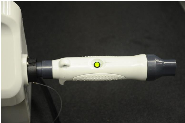
If you get a green light, power supply is good! If there is no light, the power supply should be replaced.
