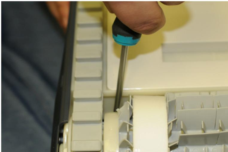
Pop the brush loose by gently prying the brush upward with the screw driver.
