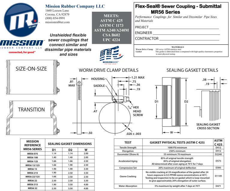
**Used to Join -** MR56 Series couplings are used to join cast iron or plastic to cast iron or plastic.
