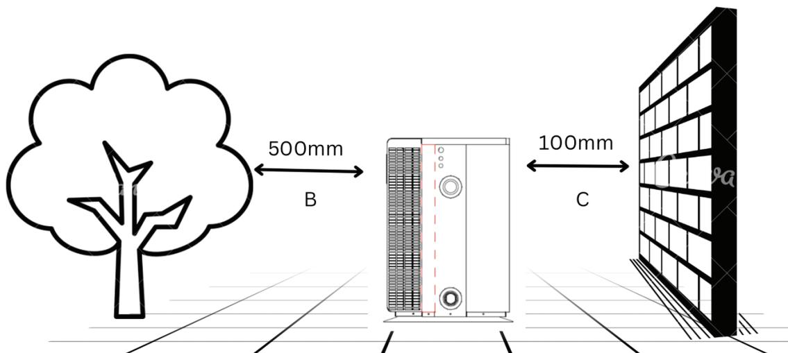
Distances used are specific to the ESV3-110 Model and are used as an example for preparing your heat pump installation site. Parameters are specific to each Madimack heat pump. Please use the specific parameters to your heat pump given in the following section to map out the heat pump installation site.
