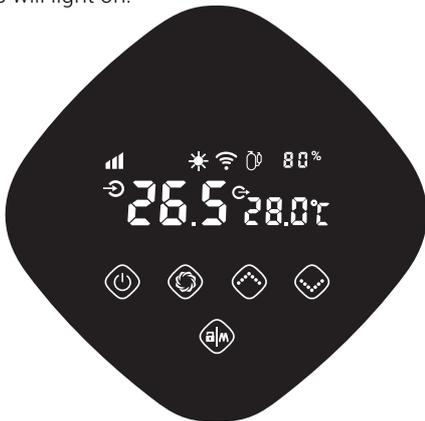
3) Press "" for 3 seconds to lock the screen; screen will be dark; lock button lights on and other buttons will light off.
