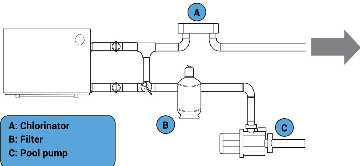
1. Chlorinator controller initiates the filtration pump either manually or through a timer.
