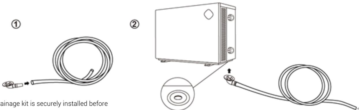
Ensure the drainage kit is securely installed before connecting pipework and electrical as it is easier to access
