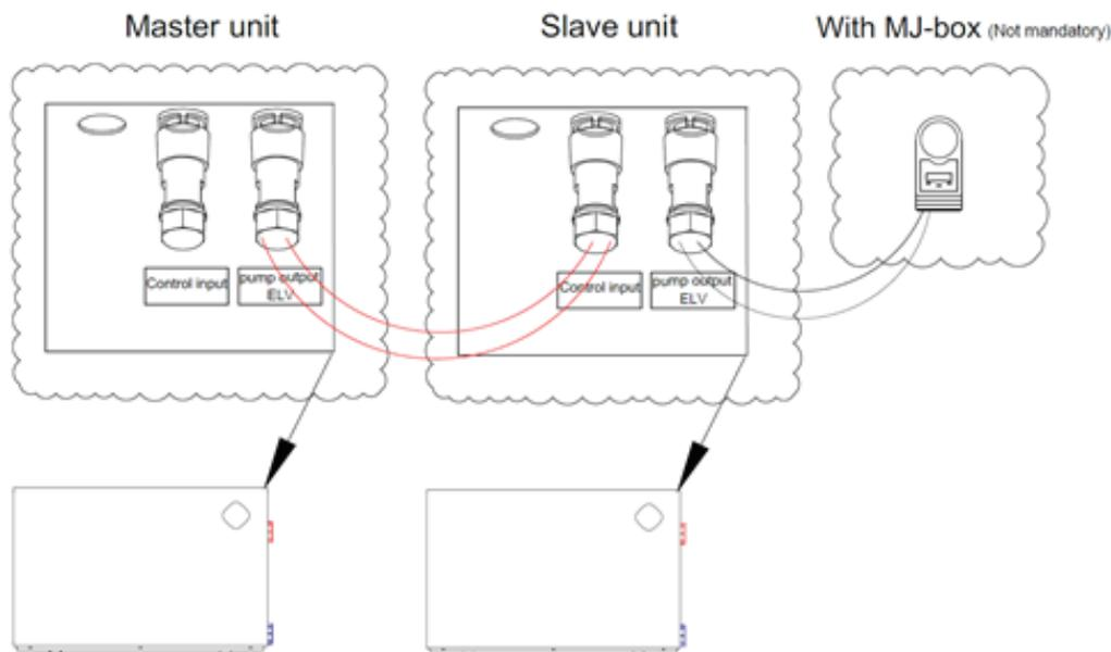
Wiring multiple heat pumps together can be achieved through a master and slave connection
