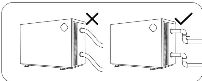
Unit inlet and outlet water pipe connections are 40 mm
