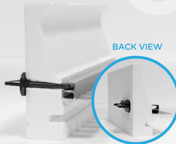
Rotate clip 90° vertically to lock it into the cover track.
