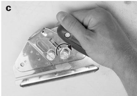
1. Loosen the right knurled knob (a) to adjust the "throat" opening (b) to the desired height for precise, variable height cuts, then tighten (c).
