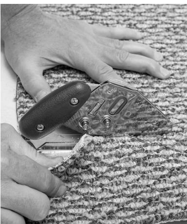
3. Place the "throat" of the cutter over the carpet so the blade and the nose of the cutter are between the rows of the carpet loops. The base allows for cutting over top of the carpet by protecting material underneath.
