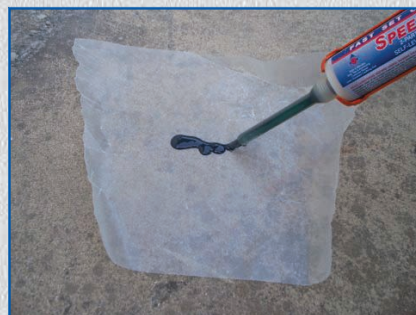
Start dispensing Speed Bond onto paper to insure good mix and flow.
