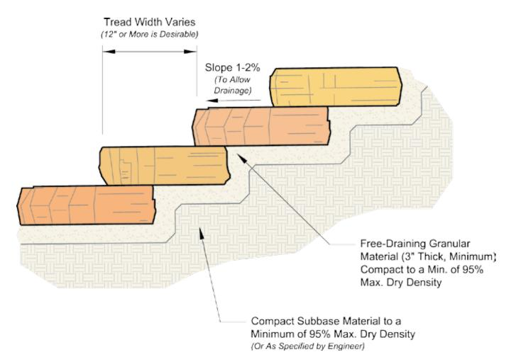
**Excavate and grade the area for the first step**. Steps should be placed on at least 3" of free draining soil, such as sand or peastone. Compact soil to a minimum of 95% Standard Proctor.
