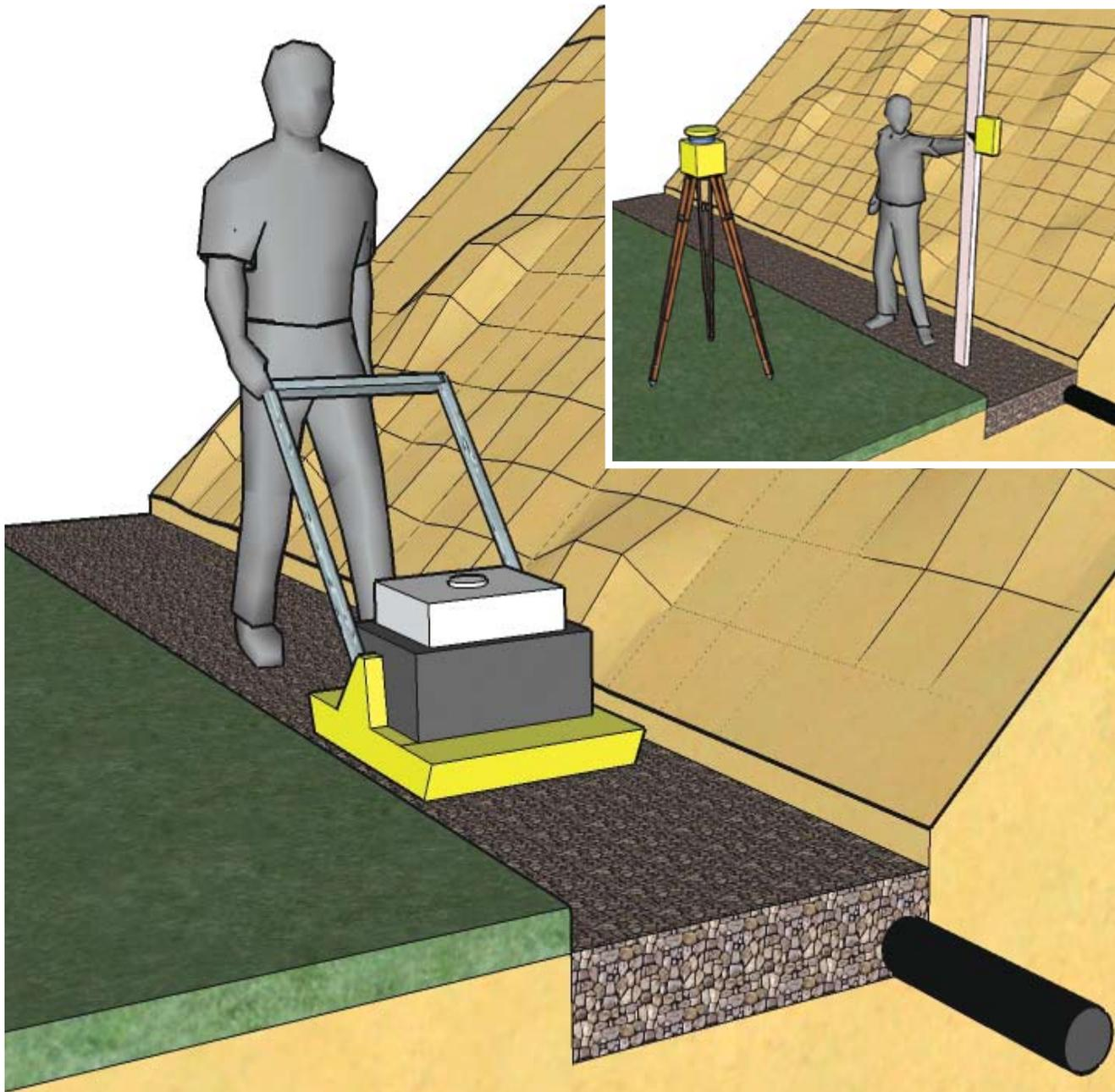
Proper base preparation is one of the most critical elements of retaining wall construction. The retaining wall is only as stable as the foundation it is placed on. If sub-base soils are deemed unstable, contact a qualified geotechnical engineer for remediation.
