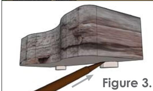
You may find it useful to **remove the shear heels from the blocks to be placed on the bottom course**. This can be done using a demolition bar. (see **Figure 3**.) Be sure to do this in a safe manner, keeping your body away from potential falling hazards.
