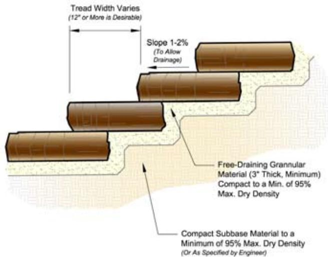
**Excavate and grade the area for first step.** Steps should be placed on at least 3" of free draining soil, such as sand or pea-stone. Compact soil to a minimum of 95% Standard Proctor.
