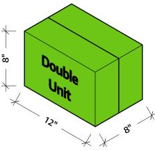
Sometimes SFUs are broken up or can't be used. The Double Unit is the next preffered unit. Double Units are grouped for strength and speed in construction. They are always represented in green.
