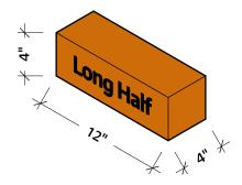
Long Halfs are simply made by cutting a block along its center on the longest axis.
