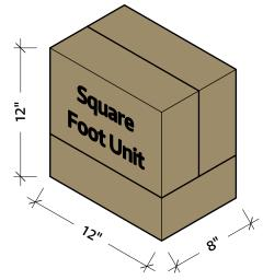
The "Square Foot Unit." consists of three block as shown. By rotating this unit (SFU) we are able to build quickly and easily while keeping bond lines broken up. These will always be shown in a tan color.
