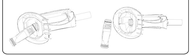
7. Remove the RETAINING RING from the DIAPHRAGM. Discard the used diaphragm.
