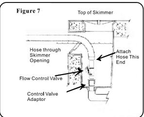
The Flow Control Valve is preset between position 3-4. This provides the ideal operating flow in most pools. But if necessary, the flow can be adjusted by using any setting from Position 1 through 6 (1= minimum flow, to slow your cleaner down, 6 = maximum flow, your cleaner will run faster). See Fig 8.
