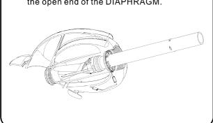
(f) Slide the THRUST WASHER over the INNER EXTENSION PIPE. The flat side (widest diameter) of the THRUST WASHER should face down.
