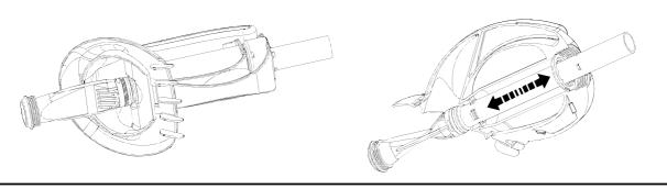
6. Twist the DIAPHRAGM, removing it from the INNER EXTENSION PIPE.
