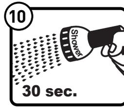
Wait a few seconds and wet the same section again for **another 30 seconds or until joint are saturated** (water can no more penetrate the sand). Avoid run-off and foaming. Check for water accumulation at the surface of the jointing sand
