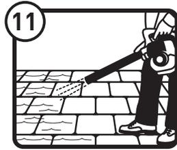
On textured pavers, use the blower to remove the excess water off the surface and into the joints.
