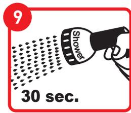
Starting from bottom of the slope, quickly shower a 200 sq. ft. section to set the sand for **30 seconds**.
