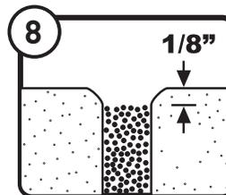
8 Sand level must be at least 1/8" below top of pavers or up to the bottom of the chamfer.
