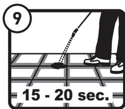
A handheld or backpack sprayer is recommended for precise watering of the joints. Using the water sprayer, starting from bottom of the slope, quickly water the joints of a **100 sq. ft. section\* (15 to 20 seconds)** by spraying over the joints. Aim to achieve complete saturation of the joint in one pass.
