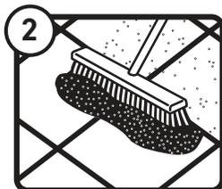
Using the street broom, fill joints completely. Spread sand over **short distances**.
