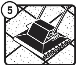
Pass the paver roller compactor over the entire surface a second time. **Multiple passes** may be required until joint saturation is reached.
