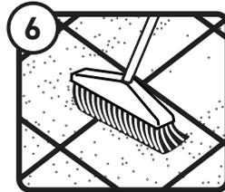
Remove excess sand from the surface with the broom.
