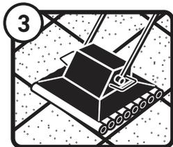
Pass the paver roller compactor over the entire surface to compact the sand.
