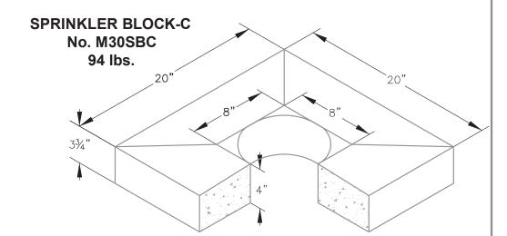
A precast concrete protector for a variety of sprinkler heads. For extra heavy duty applications where maximum protection is required. Can be set above ground or at ground level. Approximate dimensions and weight shown.
