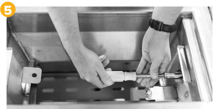
Use a 13mm socket to remove the NG orifice
