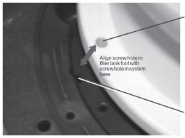
Screw hole–filter tank foot (a second such screw hole is located 180° opposite this one)
