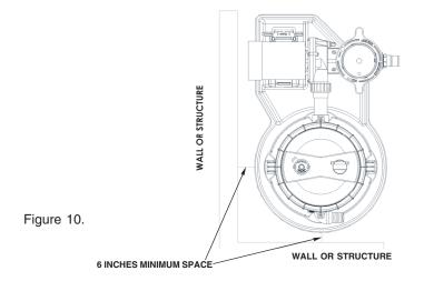
10. Provide sufficient space above the filter to remove the filter lid or for cleaning and servicing. This distance will very with the model of filter you are using. See Table 1 below for required vertical distance.
