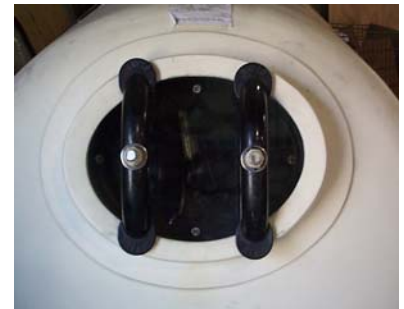
Correct yoke orientation
