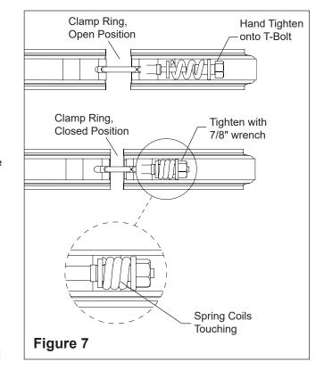
**Note:** Check the spring coils at least once a month to ensure proper tension. If spring coils do not touch then **shut off pump and relieve pressure** and tighten the nut and tap filter clamp ring until the coils touch.
