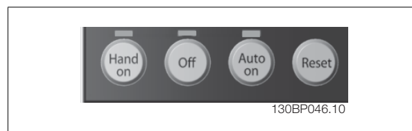
Illustration 7.5: Operation keys of the numerical LCP (NLCP)
