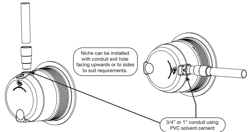
Niche can be installed with conduit exit hole facing upwards or to sides to suit requirements.
