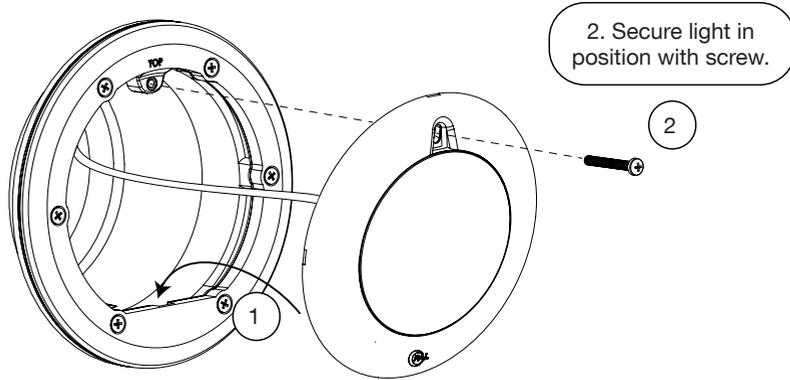
1. Rotate light onto face plate using hook.
