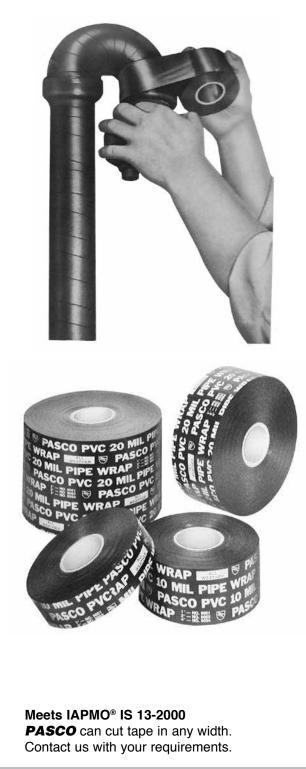
**PASCO**'s "All Weather" Pipe Protection Tape is a tough PVC plastic tape with special high tack adhesives formulated to resist corrosion. It is easy to apply by hand with no special tools or equipment. It provides positive protection against abrasion and corrosive action for steel pipe, fittings & electrical conduit systems.
