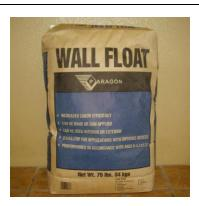
WALL FLOAT: is a pre-blened plaster mix specifically designed for the tile contractor. The control of mix ratio and quality of sand make it a superior product to job-site mixes. Wall Float is a blend of Portland Cement Type I-II-V (ASTM C 150), Lime Type-S (ASTM C 207), and washed and graded plaster sand (ASTM C 144) Specifications.
