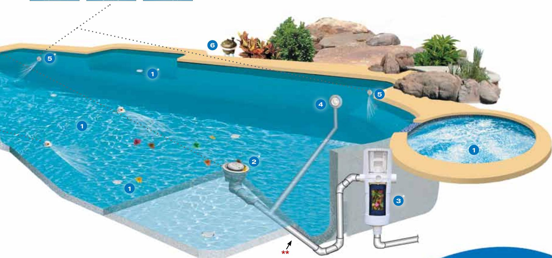
\*MDX-R3, SWINGJET, MVFUSE, DEBRIS CONTAINMENT CANISTER, AND NOZZLES IN STEPS, BENCHES, SWIMOUTS, AND SPA ARE OPTIONAL.
