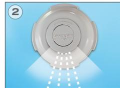
When not operating the Swingjets retract and then rotate to a new position upon the next activation.
