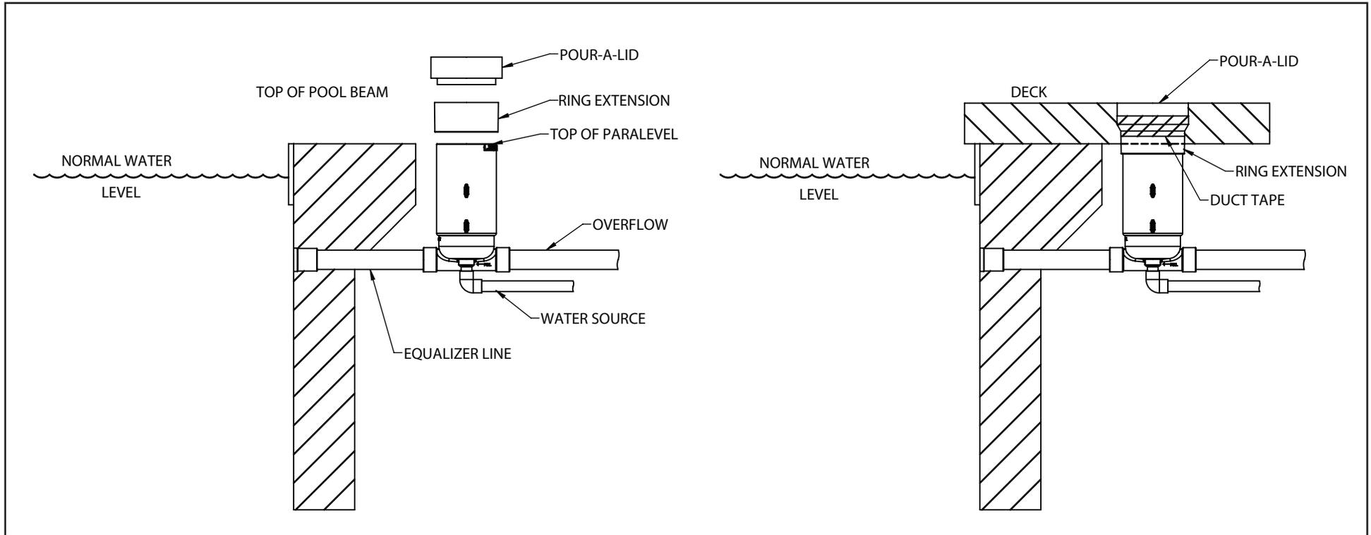
The Paramount Paralevel Pour-A-Lid will accept decks with a thickness of 2 and 3/4 inches up to 4 and 1/2 inches.
