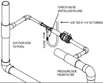
Fig. 27 **NOTE: CLEAR O3 MUST BE MOUNTED 1' ABOVE WATER LEVEL**
