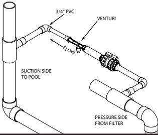
5. Connect a short piece of 3/8" OD X 1/4" ID tubing on the barbed end of the venturi.
