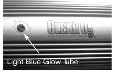
**NOTE: IF YOU SEE A RED OR YELLOW LIGHT THRU THE GLOW TUBE TURN OFF THE POWER IMMEDIATELY AND REPLACE THE LAMP. RUNNING THE UNIT WITH A YELLOW OR RED LIGHT WILL DAMAGE THE BALLAST.**
