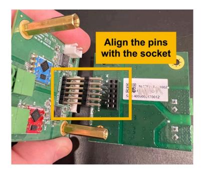
Gently push down on the top board so that the holes from the standoffs are right below the top board mounting holes. Do not use excessive force or else you could damage the connectors and possibly both Chemistry boards.
