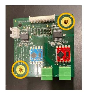
7. Use the 2 screws removed from the bottom board, and fasten down the top board to the standoff screws.
