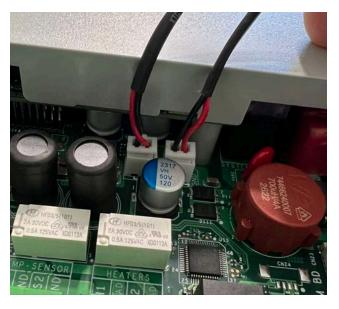
9. Once you've completed connecting the 2-pin wire, you can continue to <u>Installing the pH and ORP Probes</u>, or you can reattach the bottom cover and power The Attendant Mini back on.
