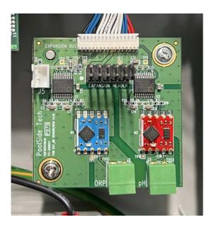
Once the Chemistry Board is securely fastened to the mounting pillars, you can continue to connect the communication wires to the main board.
