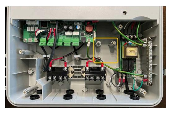
5. Install the Chemistry Module by **gently** placing the board over the area and **holding** it in place while inserting and tightening the mounting screws (included). Be careful **not to over-tighten** the screws!
