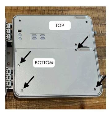
4. Locate the Chemistry Module mounting pillars near the center of the compartment. See image for placement.
