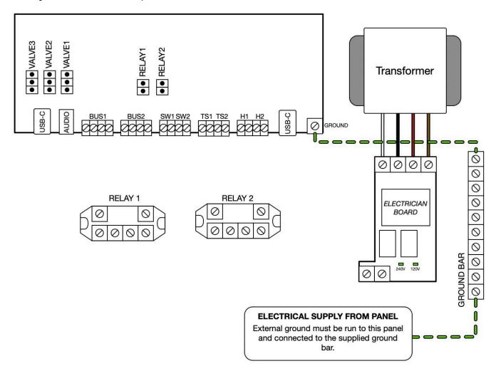
This bottom portion of the controller contains all of the **high voltage** relays. The high voltage relays connect to the main circuit board by red/black wire to the board connectors labeled **RELAY1-2**.
