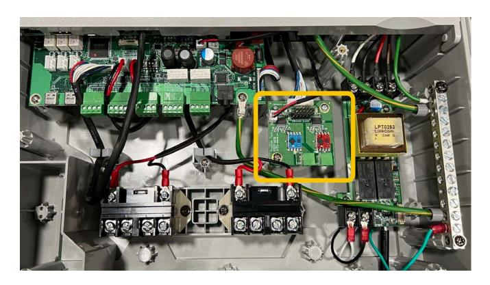
5. Next, you will need to **remove** the two crosshead screws that are currently installed on the first Chemistry board - the "bottom" one and **replace them with the 2 standoff screws** provided with the Dual Chemistry kit. Use a small wrench or 5mm socket to gently tighten each standoff. Do not over-tighten!
