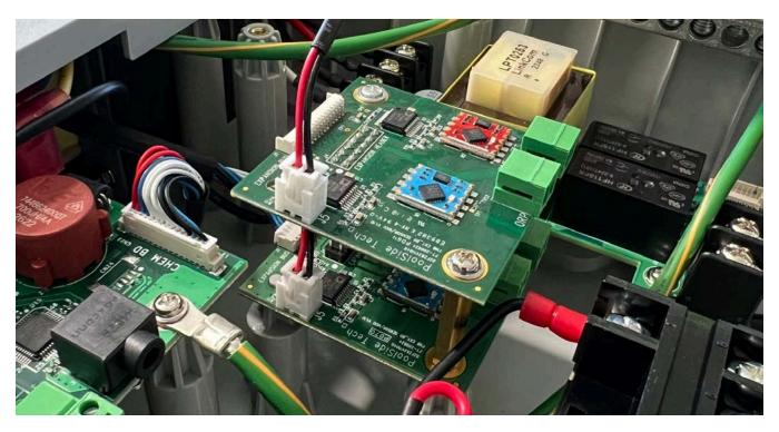
8. Next, take the 2-pin cable and connect that to the **GPIO2** socket on The Attendant Mini.
