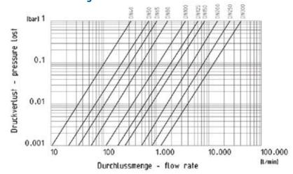
Measurements implemented as per DIN EN 60534-2-3 Valves in pressure loss diagram obtained at max. opening angle with PVC 145 psi pipes and flow medium water at 20°C/68°F.
