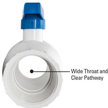
The solid one piece handle can be easily removed or replaced without tools. The 1" internal and 1 1/2" external hex shape of the stem allows the valve to be operated with a wrench or socket if the handle is removed.
