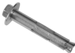
Sleeve Anchors: Similar to the wedge anchor. It can be used in the same materials as the wedge anchor, but can also be used in soft concretes because the compression load can be distributed over a longer length. Can be installed through the fixture. Assemble nut and washer on stud and insert into predrilled hole. Anchor is hammered into hole until the nut is seated. ICBO approved
