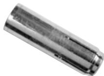
Drop In Anchors: This steel anchor performs well in a variety of concrete strengths. Can be used in brick. Any head style screw can be used. The screw can easily be removed or loosened and retightened. Drill hole in concrete and drop anchor into hole. Place setting tool over anchor and hammer until set. ICBO approved.
