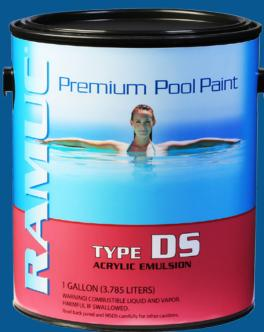
**Type DS** offers advantages over traditional solvent-based paints. DS Acrylic can be applied to damp surfaces and previously painted chlorinated and synthetic rubber surfaces. Use of DS allows the pool to be filled within 3 days after the final application of paint. Acrylic coatings such as DS are used when short down times are critical. Water-based acrylics are extremely color-fast and UV resistant.
