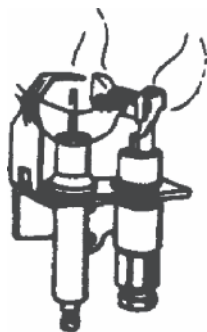
Fig. 2: Pilot Burner Flame
