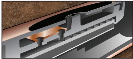
XFS emitters are protected from root intrusion by Rain Bird's patent-pending Copper Shield Technology resulting in a system that does not require maintenance or replacement of chemicals to prevent root intrusion. The copper color outside ensures the copper chip is inside.
