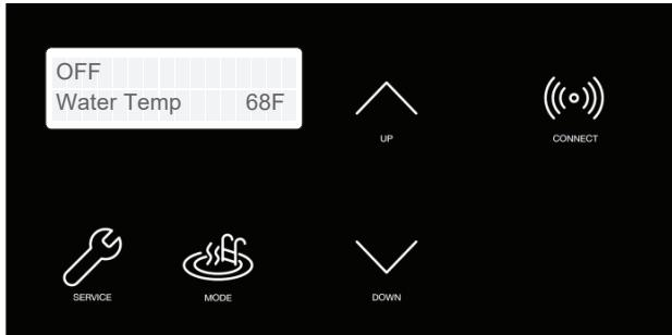
Figure 106. Wi-Fi Reset – Press and Hold CONNECT
