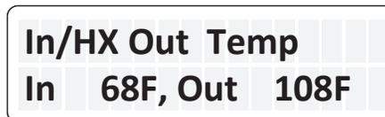
Figure 41. Inlet and Heat Exchanger Outlet Temperature
