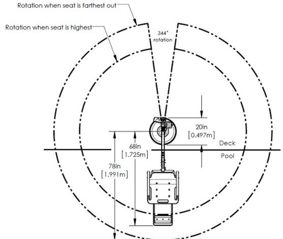
This fixed anchored lifting system can be installed in an existing round anchor.
