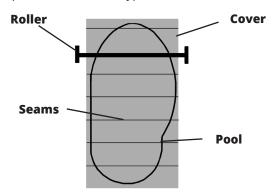
When cutting the cover, allow a 1" wide border around the pool edge to compensate for shrinkage.
