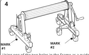
Using one of the two holes in the Frame as a guide, make mark #1 on the deck. With a 1/2" concrete drill bit, drill a 1 1/2" deep hole at mark #1. Complete steps 5 and 6 before continuing with step 4.
