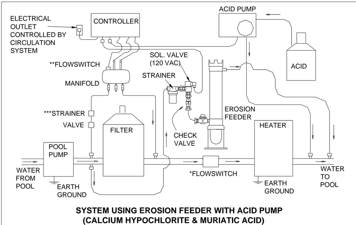
\*SAFETY FLOWSWITCH FOR PROTECTION OF HEATER AND TO ENSURE DILUTION OF CHEMICAL INTO POOL.
