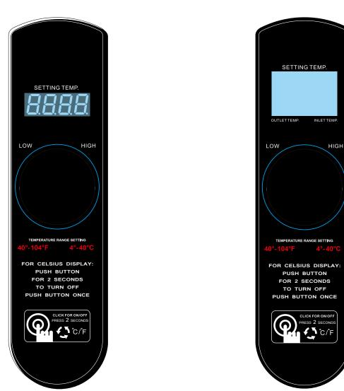
Figure 3. Digital Control for Models ELS 0005 and 0011
