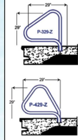
**Cross Braced Return-to-Deck Rails (3 & 4 Bend)**
