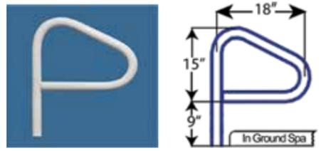
For Core and Anchor Socket Mounting
