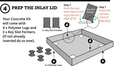
Set the Inlay Lid (C) face-up on a flat work surface away from the main slab pour area. To achieve a seamless finish, the Inlay Lid should be filled with the same concrete mix poured directly around the skimmer box.
