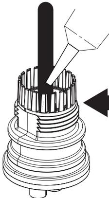
FILL BACK OF CONNECTOR BARREL WITH LANOLIN UP TO THE INDICATED POINT.
