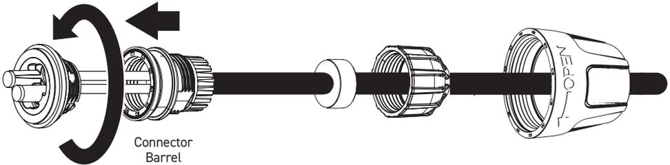
LEAVE THESE PARTS DISASSEMBLED UNTIL AFTER ADDING LANOLIN.
