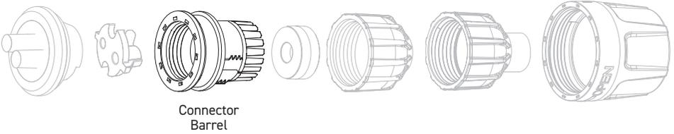
FEED THE CONNECTOR BARREL ONTO THE CABLE.
