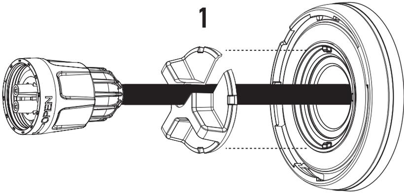
LOOSEN BY HAND UNTIL THREADED COLLAR IS COMPLETELY UNTHREADED.
