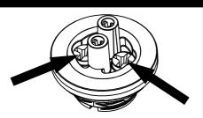
USE A MANUAL PHILLIPS HEAD SCREWDRIVER TO ENSURE THAT THE 2 SCREWS INDICATED ARE FULLY SEATED. PROCEED TO STEP 6.
