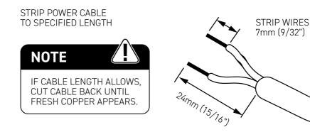
2 START ASSEMBLY OF CONNECTOR PLUG
