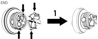
**2:** FEED THE TWO STRIPPED CABLE ENDS THROUGH THE TWO HOLES IN THE BACK OF THE SCREW TERMINAL END
