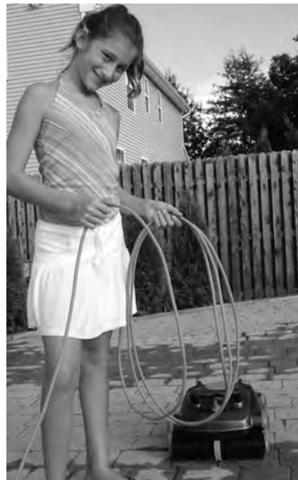
Hold the cord close to the cleaner. Make a roughly two foot loop with the cord as shown.
