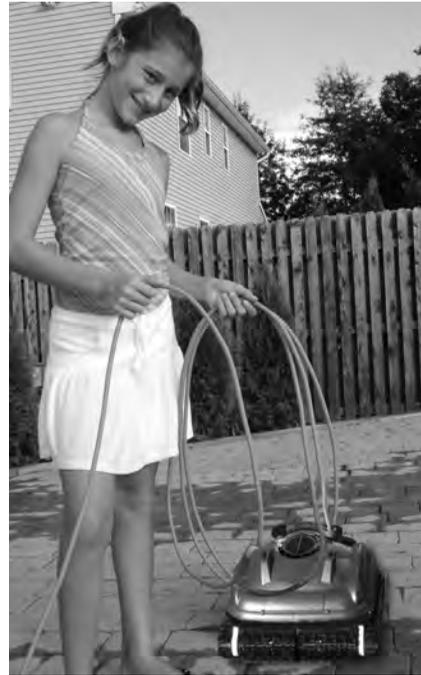
Hold the cord close to the cleaner. Make a roughly two foot loop with the cord as shown.
