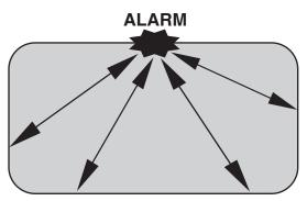
Place alarm in a central location for shortest distance from all parts of the pool.
