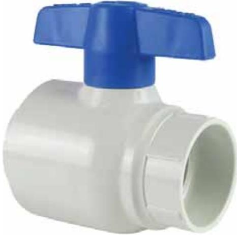
A high quality, economical quarter-turn shutoff valve designed for irrigation, pool and spa, and general purpose applications. IPS sizes 1/2" - 2" available in PVC White, PVC Gray or CPVC with socket or threaded end connectors. Sizes 3" - 4" available in PVC White with socket or threaded end connectors. 6" size available in PVC White with socket end connectors and high-efficiency lever style handle for easier operation.
