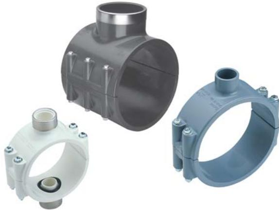
Spears® PVC & CPVC Clamp-On Saddles allow quick, easy and reliable addition of branch lines to existing piping system lines. These versatile saddle units can be used in either temporary or permanent installations on all types of pipe with IPS (Iron Pipe size) outside diameter, such as PVC, CPVC, Polyethylene, Polypropylene and Steel.
